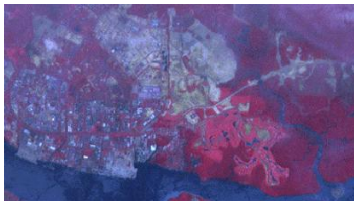
Figure (4) : Multispectral SPOT image of the same area with Radiometric and geometric corrections and transformed map projection (UTM projection).
